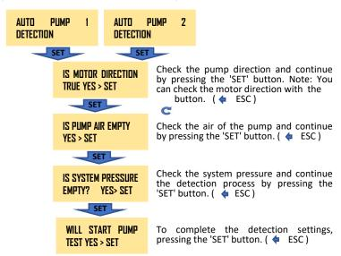
**NOTE:** During the test process, the controller will start the motors for 3.5 seconds and the system will give one of the following responses. Continue your operations according to the response given.
